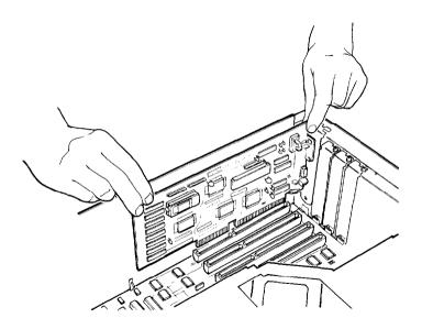
6. Insert the card into the slot, guiding it straight down. Once the connectors reach the slot, push the card downward firmly (but carefully) to insert it fully. You should feel the card fit into place.
